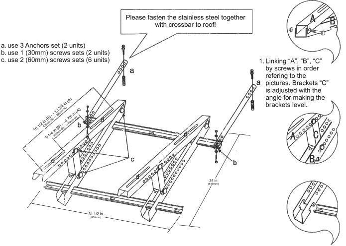
Optional: Plece the Vibration mounts on "d" (total 4 position). Install the Vibration mount using 1 (30 mm) screws sets.
