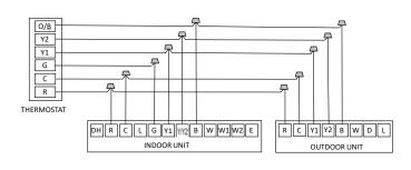
• Wiring for 3H and 2C thermostat
