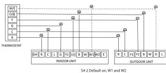
shorted for single stage Aux heat operation. Turn off to separate stages.
