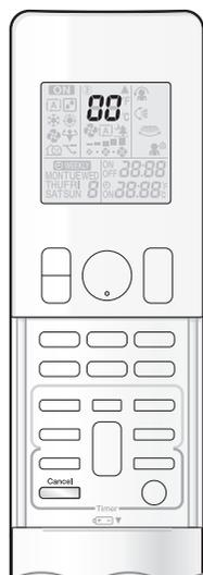
1. When **Cancel** is held down for about 5 seconds, “00” blinks in the temperature display section.
