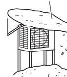
Install the unit high enough off the ground to prevent burying in snow.
