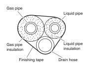
• Be sure to insulate both the gas and liquid piping and observe the insulation dimensions as below.
