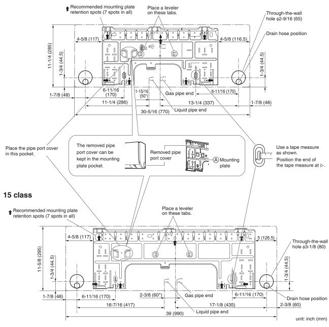
\* Depending on the model, the actual distance between the liquid pipe end and gas pipe end may differ from the distance between those symbols on the mounting plate (the distance listed in this manual).
